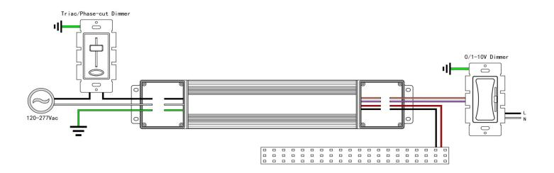
1. Input cable 3\*18AWG, the Green cable to GND, Black cable to L, and White cable to N of Mains AC.
